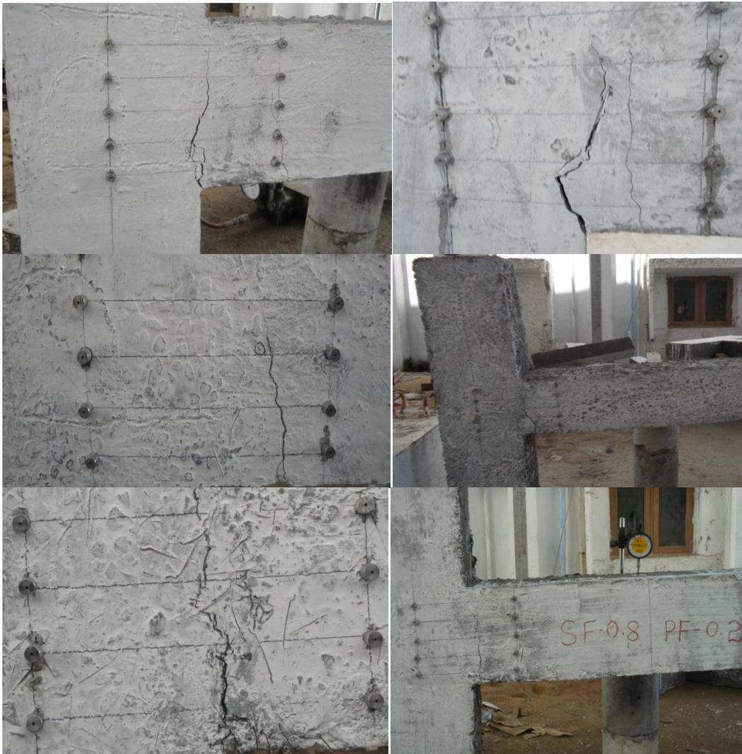
Figure 9. Crack pattern of beam – column joints specimens after failure
