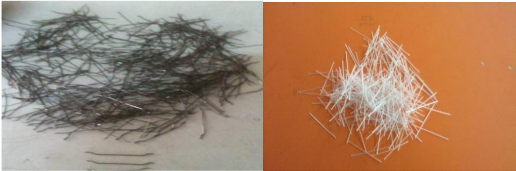
(a) Hooked end steel fiber (b) Polyolefin straight fiber
