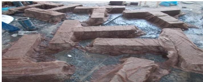
Figure 4. Gunny bag curing of specimens
